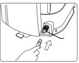
Min. length/i.d. of hose: 20 ft, ½". Clean water inlet screen at least monthly Max. inlet water pressure 150 psi.
